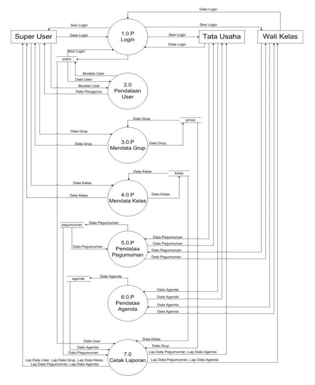
Figure 4.6 Data Flow Diagram (DFD) Level 2 Agenda Announcement Autopost System
